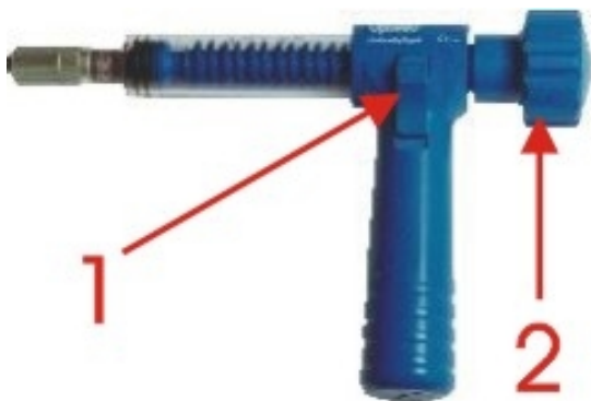
Fig 1m: PC Cemento® set pressure gun 1-quick release lever (immediate stopping of the injection) 2- Screw applicator, pressure resistant
